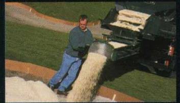
Cross conveyor with swivel action quickly fills bunkers and back fills trenches.
