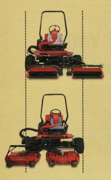
Toro® Groundsmaster® 3500-D and Reelmaster® 3100-D: Two innovative trim mowers with the Sidewinder™ cutting system. The reels on the 3100-D and the ground-following rotary decks on the 3500-D move side to side for superior trimming.
