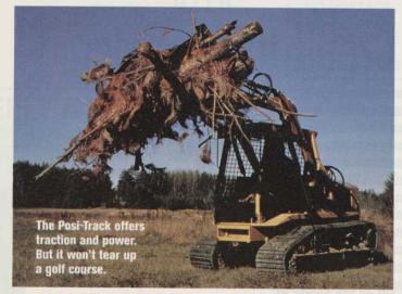
cause too much damage. But Cope discovered that the Posi-Track's intricate wheel pattern within the rubber-tracked undercarriage not only gave the machine a light footprint, but also traction and power.
