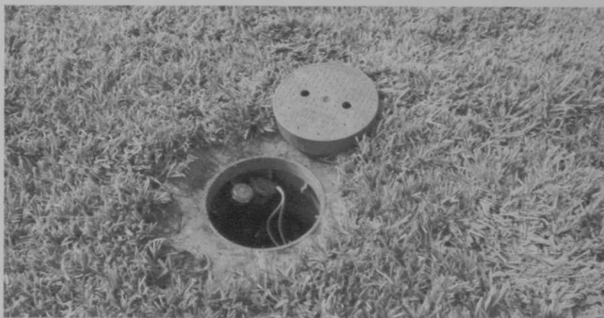
A tensiometer is shown, installed in St. Augustinegrass turf. The tip is located four inches below the turf surface. The tensiometer is wired in series to the solenoid.
