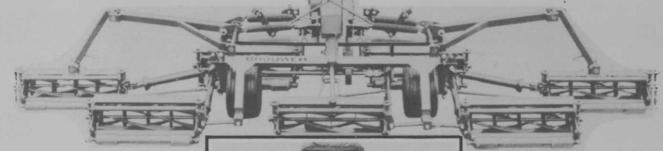
Run a 7 gang unit, cut up to 7 acres per hour with a 30 HP tractor
