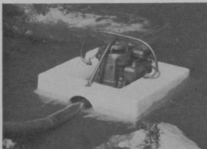
Barebo has floating evacuation pump
