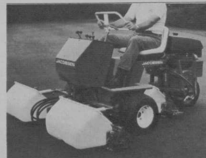
New mower back-laps in place
