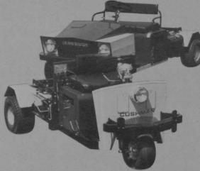
add any of the Turf-Truckster's accessory pieces, thanks to Cushman's pindisconnect system. No bolting, no hitching. Just snap two or three pull pins in place and you're ready to hit the turf.
