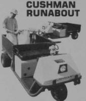
Moving people and equipment efficiently is what the Runabout is all about. The two-man 18-hp model has a 1,500 pound payload capacity and, like the one-man 12-hp Runabout, features a  $4^{1/2}$ ' pickup box and 3-speed synchromesh (2nd & high) transmission. And both deliver plenty of maneuverability, without tying up a golf cart that could be turning a profit on the course.
