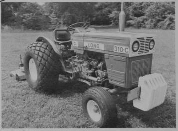
**310-C:** A 2-cyl. compact, 28 PTO H.P. tractor. Standard features include: Continuous PTO, 6-speed trans., 3-pt. hitch with draft and position control, and more. Hydrostatic steering optional. Excellent turf or small farm tractor. Turf or general purpose farm tires. Wt. 3,159 lbs. (approx.). Price with 5.00 x 15/12.4 x 24 GPF Tires.
