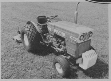
**260-C:** This compact 24 PTO H.P., 2-cyl. diesel includes as standard equipment: Continuous PTO, 6-speed trans., 3-pt. hitch with draft and position control, and more. Hydrostatic steering optional. The perfect tractor for turf and horticultural work. Wt. 3,180 lbs. (approx.). Turf or general purpose farm tiresPrice with 5.00 x 15/12.4 x 24 GPF Tires. LIST PRICE\*\*: 2-WD — \$5,525.00
