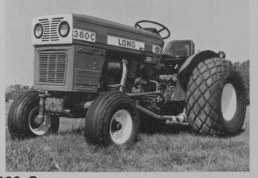
**360-C:** A heavy-duty, compact 3-cyl., 35 PTO H.P. tractor engineered for outstanding performance and economy. Standard equipment includes: 6-speed trans., hydrostatic steering\*, continuous PTO, 3-pt. hitch with draft and position control, and more. The ideal tractor for heavier turf work or small farm chores. Turf or general purpose farm tires. Wt. 3,630 lbs. (approx.). Price with 5.00 x 15/12.4 x 24 GPF Tires. LIST PRICE\*\*: 2-WD — \$7,204.00
