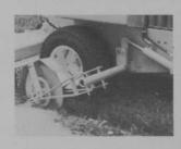
A side-mounted edger has been added to the line of attachments for Excel Hustler mowers. The new edger consists of a single concave coulter
