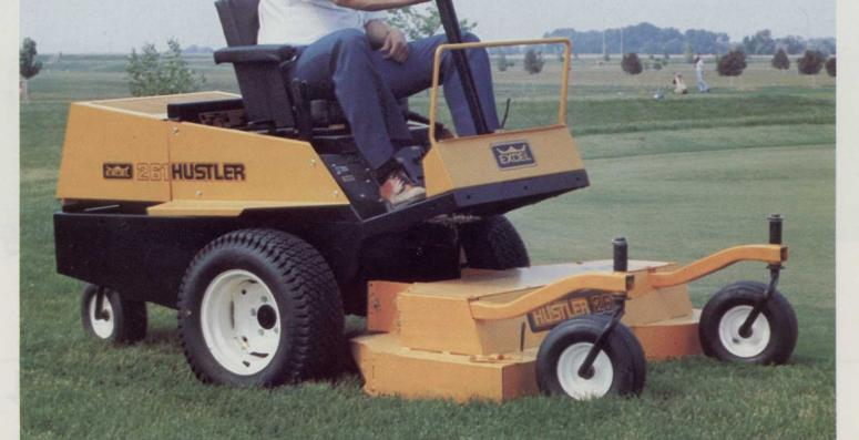
There's Mower: Belt drive runs straight from B&S 2-cylinder engine to mowing deck mounted on the same floating frame. No twists to steal power or wear out belt. Shorter wheel base to mow evenly, reduce scalping. Tractor comes with 3-way deck, full safety group.
