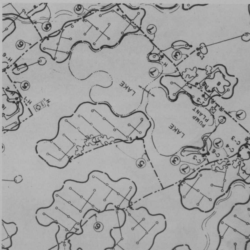
This portion of an irrigation system plan layout shows head and piping layout.
