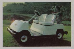
• The Yamaha gas car has an automatic fuel-oil mixing, solid state ignition and a lean burn fuel system – all features that cut fuel consumption and reduce maintenance.
