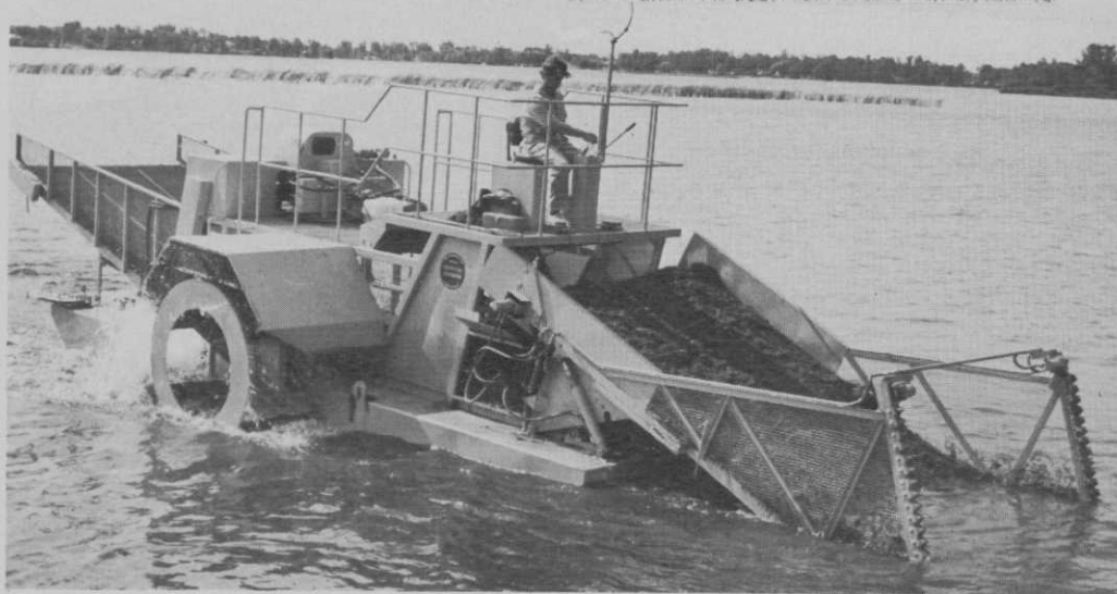
Mechanical harvesters of aquatic weeds are usually too large for all but the largest golf course lakes, but fish such as the white amur can effectively control aquatic weed growth where legal.
