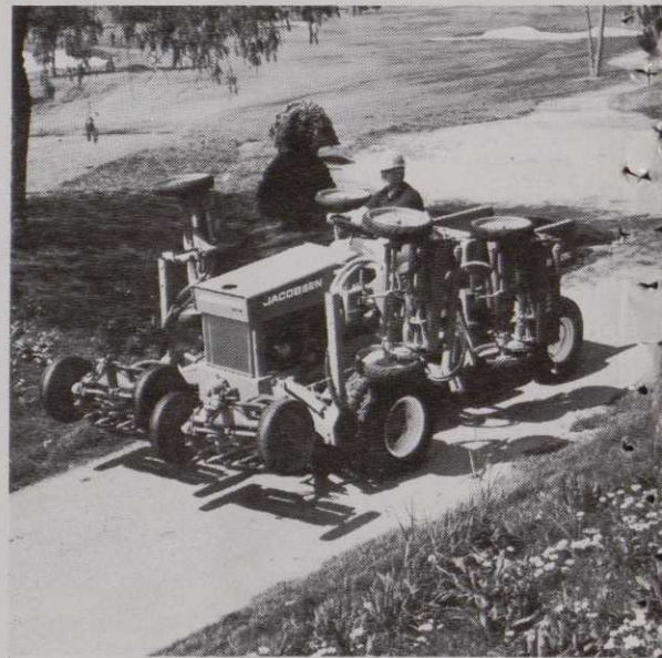
The advantage of hydraulic lifts on fairway and rough mowing tractors is not so apparent in mowing as it is in transporting the mowers from one part of the course to another. The operator doesn't even have to get off the tractor.
