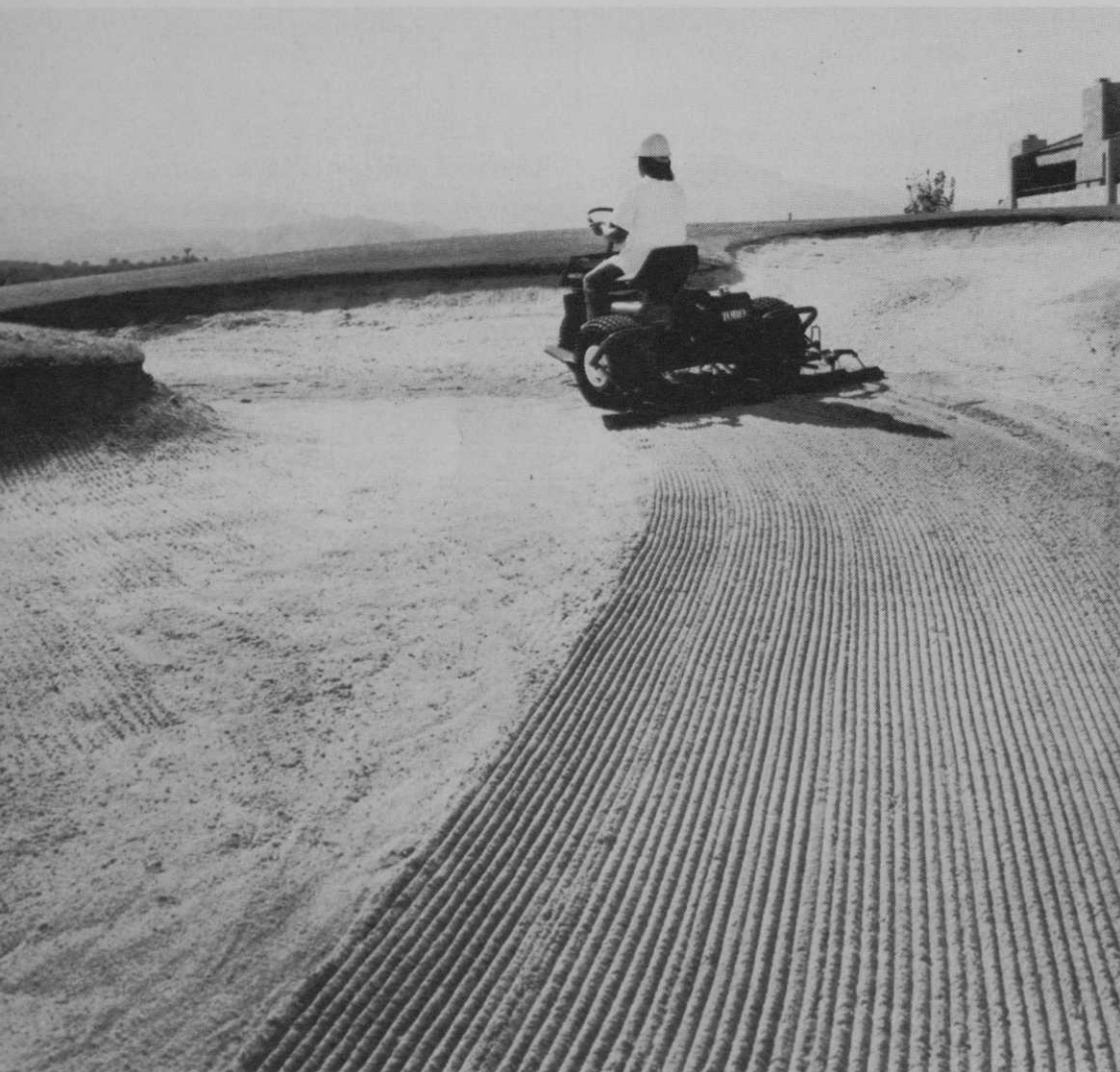
Like the one pictured above, the traps at the Country Club of Colorado are well-groomed by one worker using a Toro Sand Pro motorized trap rake.
