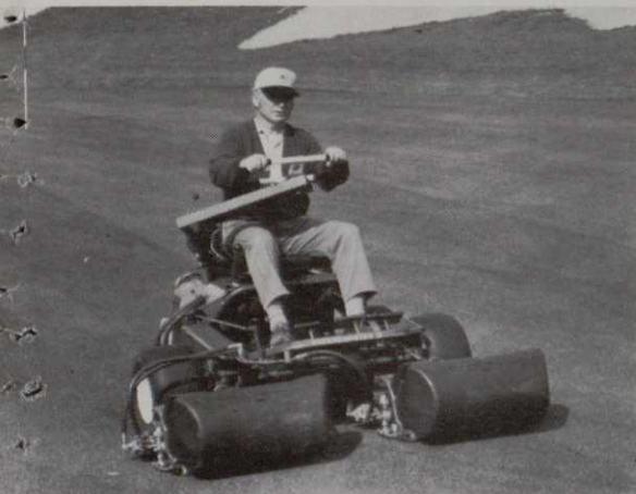
Greens at the Country Club of Colorado are mowed by a triplex mower like this Toro Greensmaster 3.
