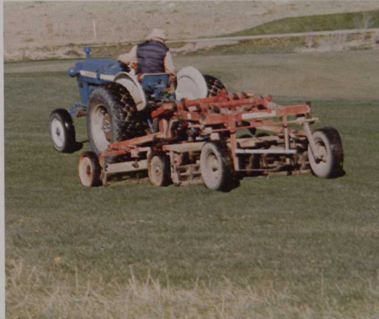
Five-gang mowers cut the rough at the Country Club of Colorado, making it a one-man job.
