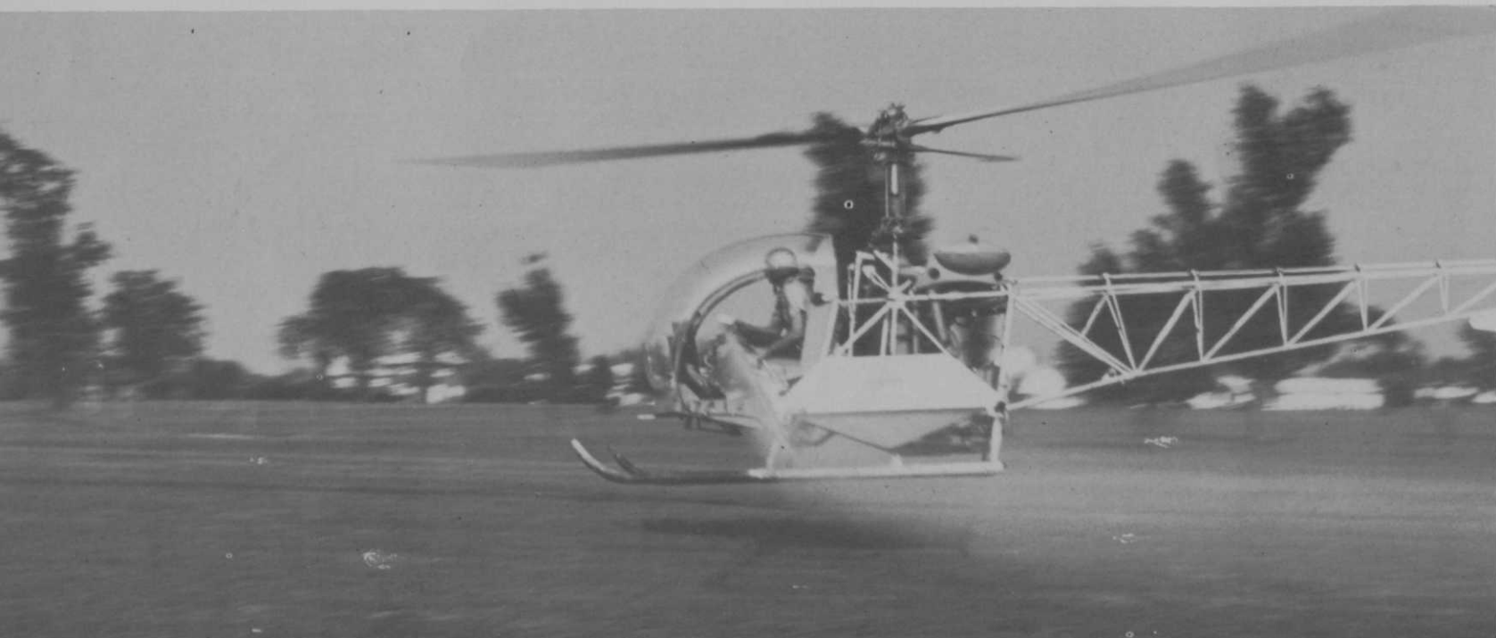
LEFT: Spray nozzles are carefully checked out before takeoff. BELOW: The helicopter flies at 60 mph about 5 feet off the ground when spraying a golf course.
