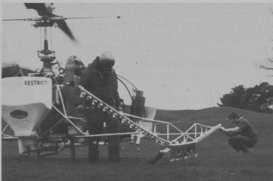
LEFT: Spray nozzles are carefully checked out before takeoff. BELOW: The helicopter flies at 60 mph about 5 feet off the ground when spraying a golf course.
