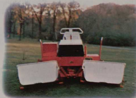
The mowers are fully articulated so they hug the contours of uneven ground.
