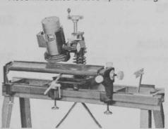
Foley's Bed Knife Grinder Foley's Bed Knife Grinder provides exact angles for precision sharpening. Grinds bed knives and straight knives
