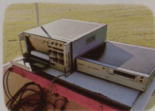
Engine and reel RPM's are monitored by the readout device on the right and fed to the strip chart recorder on the left which continuously prints out data.
