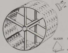
INDIVIDUAL SLICER OR SPIKER UNITS SHOULD BE ATTACHED TO DRUM SURFACE.
