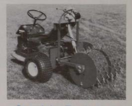
Specialty Equipment Even a vehicle built for specific use, can be used with the Dedoes aerator to give quick, neat aeration for small areas.
