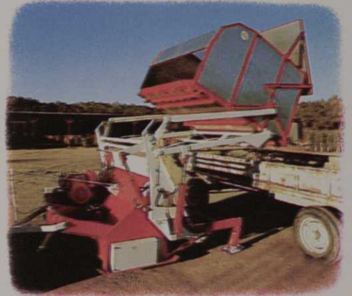
Hydraulic dumping feature of HL models can dump at any height up to 8½'.
