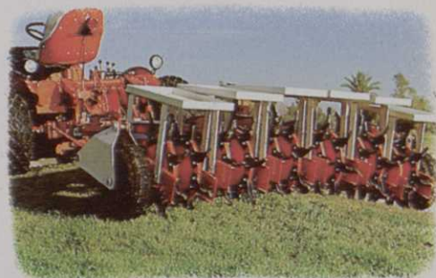
Notice how each section rides close to uneven contours of ground to provide even aeration. Individual weight trays provide pressure.
