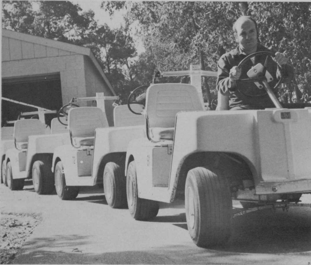
Bethpage's golf cars are moved from storage shed to pickup station in trains of six. Front car easily pulls the train.
