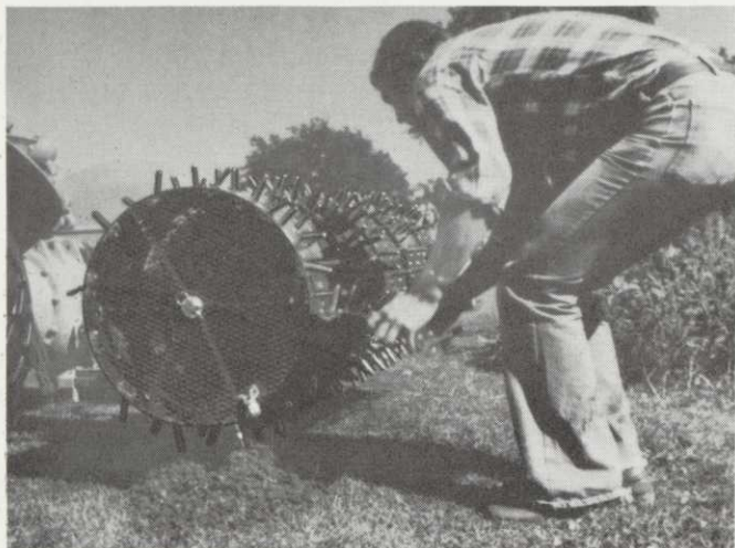
TCA-601 Supreme with conversion unit — 180 tines (300 if necessary). Has hinged door and removable sides. Collects plugs internally or can be used same as standard model.
