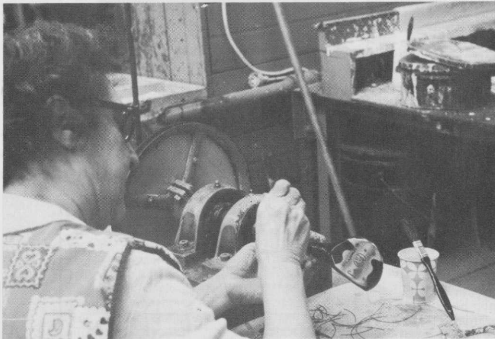
Applying winding by hand is just one of several hand production methods done on each Spalding wood. Shown above is work being done in the custom order department. Between 50,000 and 60,000 pieces passed through this department last year. Most employees in the section have at least 25 years with the firm.
