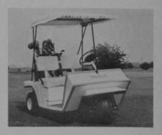
Melex. Electric, \$1,600; length, 98 inches; width, 48 inches; weight, 1,050 pounds with batteries; four wheels; steering wheel; steel body and frame. WARRANTY, both models: one year on all parts. OPTIONAL FEATURES, both models: radio, head and taillights, horn, cigarette lighter, storage box. STANDARD FEATURES: canopy, seat brake.
