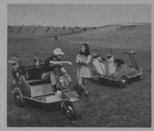
fiberglass body with steel frame. WARRANTY: 90 days on all factory defects. OPTIONAL FEATURES: canopy, head and taillights. STANDARD FEATURES: metal flake finish, beverage ice cooler.
