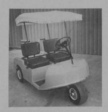
Capri-100. Electric, \$1,465; length, 93 inches; width, 45 inches; weight, 900 pounds with batteries; three wheels; tiller or steering wheel; fiberglass body. WARRANTY: one year against defective parts and workmanship. OPTIONAL FEATURES: top wheel covers. STANDARD FEA-TURES: safety reverse switch, automatic brake release, wrap-around bumper built into frame, automatic rear body latch and cushioned brake to prevent turf damage.
