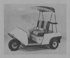
437. Electric, \$1,395; length, 911/2 inches; width, 471/4 inches; weight, 965 pounds with batteries; three wheels; steering wheel; steel body and frame. WARRANTY, both models: one year on parts and workmanship; two-year guarantee on speed control. OPTIONAL FEATURES, both models: customized cars available. STANDARD FEATURES, both models: canopy, batteries and charger and brakes on each rear wheel.
