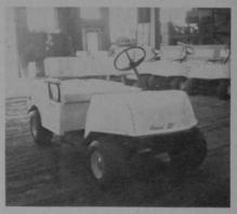
steering wheel; fiberglass body with steel frame. WARRANTY: one year on workmanship. OPTIONAL FEATURES: canopy, windshield and heater. STANDARD FEATURES: the use of propane fuel only.
