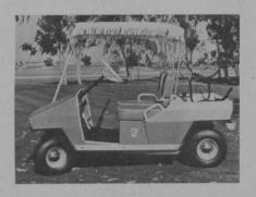
bumpers, cooling fan and cigarette lighter. STANDARD FEATURES, both models: Uni-Spring suspension system, utilizing heavy-duty leaf spring suspension integral with front and rear axles.
