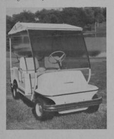
Model D-4. Gas, \$1,614; length, 100 inches; width, 451/4 inches; weight, 798 pounds with fuel; four wheels; tiller; fiberglass body and steel frame.
