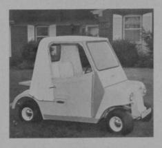
Caroche Islander. Electric, \$1,840; length, 93 inches; width, 451/2 inches; weight 890 pounds with batteries; four wheels; steering wheel; fiberglass body and aluminum frame. WAR-RANTY: one year with a two-year pro-rated warranty on batteries. OP-TIONAL FEATURES: hardtop cab with front and rear safety glass windshields, doors and side curtains, hydraulic wheel brakes, mechanical braking system on rear brakes, head and taillights and dashboard.
