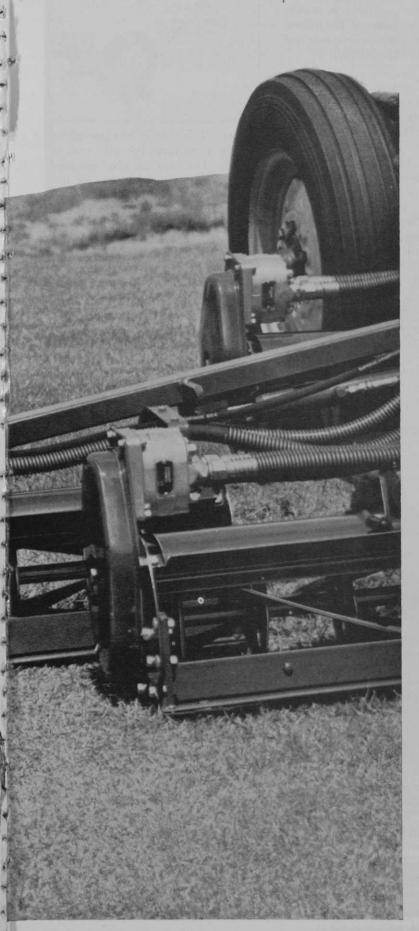
The Ransomes Hydraulic 5/7 has a proven record of high work output. Why? Because it is totally hydraulic—totally! Every part of the cutting action is controlled from the tractor seat—raising and lowering of the units, forward and reverse drive of the reels. Hydraulically powered reels allow you to cut tougher grass—easily, saves turf damage.
