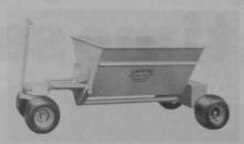
The Champion Company offers three models in its Doo-All Trailer line. Roll-Dump hoppers, available in one-cubic-yard and two-cubic-yard capacities, are also featured on two models. The third model will show the small chassis with the interchangeable flat bed in place. All units feature Terra-Tires. The two-cubic-yard chassis has a new square tongue for added strength for sharp turns under heavy load.
