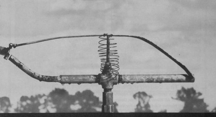
You're looking at the first Rain Bird sprinkler ever built. It was 1933 when we took the wire binding from a broom handle, welded a flat piece of copper to a length of pipe—and came up with the famous spring-actuated, impulse sprinkler that has made irrigation history around the world.
