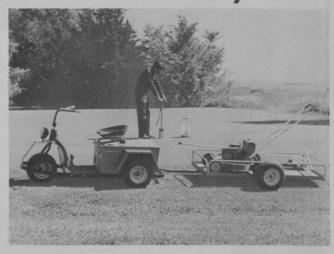
Economical but rugged low-bed trailer with big turf tires. Bed size 35" wide by 66" long with a 250 lb. load capacity. Easily holds several large trash containers, or 2 hand mowers, plus rakes and shovels or whatever equipment is needed at the work site. We'd like to send you information about these new products and the complete Cushman Turf Care System. Let us prove its performance and savings. Drop this coupon in the mail today.
