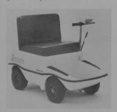
Auranthetic Corp. introduces the Mark 30, an electronically operated industrial vehicle. The new car features a transistorized-proportional speed control unit, forward and reverse, dynamic breaking and direct chain drive. The fiberglass car is
