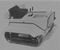
Struck Corp. announces the Mini-Dozer, a heavy-duty bulldozer with a 12hp electric start engine. The dozer features new mud design fenders, a heavy-duty clutch system and has extra-strong 10-guage steel interlocking track shoes. A quick-reversing transmission permits 360-degree turns in the unit's own length. The dozer comes in an easy-to-assemble kit form and retails for \$698.95 complete.
