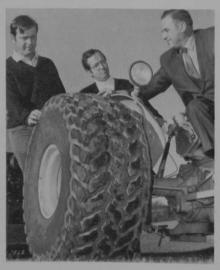
Firestone Tire & Rubber Company introduces the new Turf & Field rear tractor tire designed for golf courses, where damage to turf, particularly in sloping areas, has been a problem. The tire is 21½ inches wide with a low-profile design to provide traction while giving the floatation needed to prevent cutting and chunking of turf. The tire is designed for use on standard one-piece wheels.
