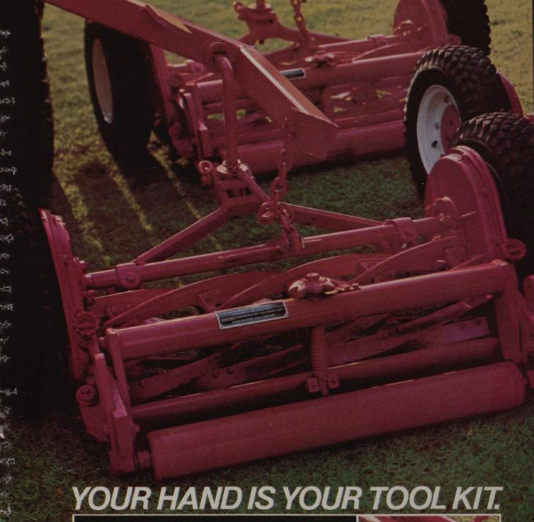
Toro's Spartan®7 gang mower gives you more cutting time, by reducing your adjustment time up to 75%. A single knob adjusts the bedknife to the reel, easily, without tools. Increased structural rigidity allows it to hold the adjustment longer, and lowers maintenance costs.
