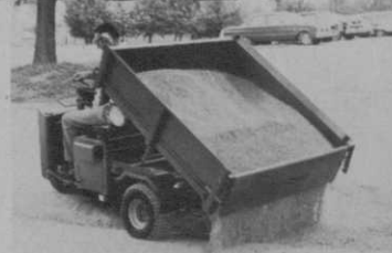
Big Box Model dumps manually. Meters out the material at correct flow. Swinging tailgate is operable from driver's seat.
