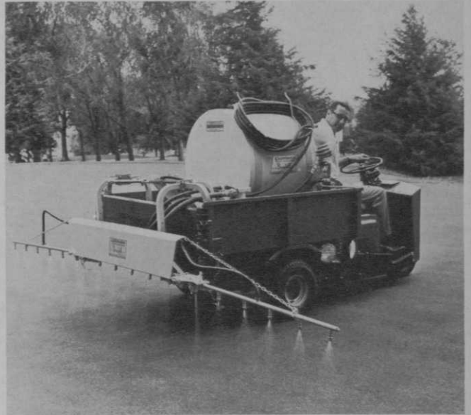
Complete Greens Sprayer shown mounted on Big Box model. Six-speed dual-range transmission and variable speed fast-acting governor assure uniform ground speed over varying terrain.
