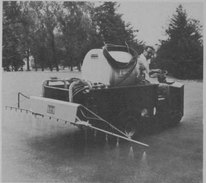
Complete Greens Sprayer shown mounted on Big Box model. Six-speed dual-range transmission and variable speed fast-acting governor assure uniform ground speed over varying terrain.
