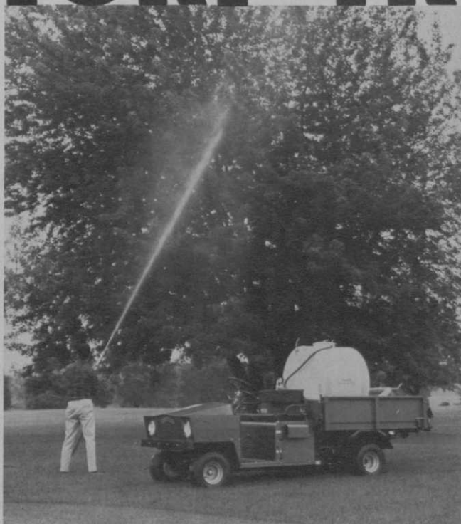
Handgun is standard equipment with Fairway Sprayer. Optional equipment with Greens Sprayer. Can be adjusted for direct stream reaching 45 feet high. Ideal for spraying ornamental trees and inaccessible areas. Excellent for mosquito control.
