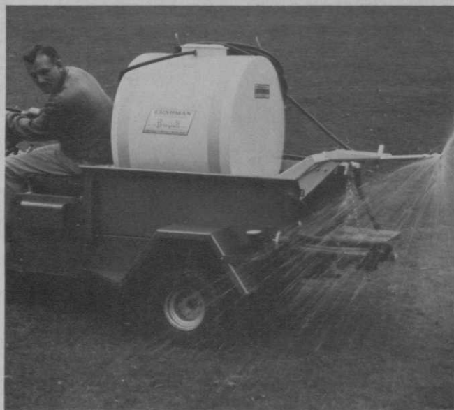
Fairway Sprayer on the Pickup Model Turf-Truckster sprays a 30-foot wide swath. Boomless nozzle, handgun assembly and 50 feet of hose are standard.
