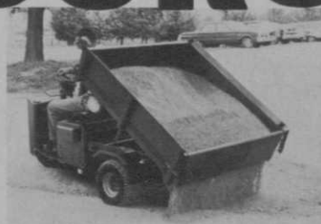
Big Box Model dumps manually. Meters out the material at correct flow. Swinging tailgate is operable from driver's seat.
