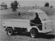
Cony America offers Cony 360, a turf maintenance truck featuring low-pressure, wide-profile tires, heavy-duty transmission with four synchromesh forward speeds and a turning radius of less than 13 feet. A flat bed is provided with removable drop panels on both sides and the rear. Under \$1,500 at coastal ports.
