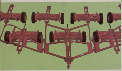
Toro offers you three **Spartan** frames to match your mowing needs. Toro Universal Frame connects to any standard tractor. It's available in 3, 5, 7 and 9 gang units. Mows fast without bouncing. Yields to ground undulations.
