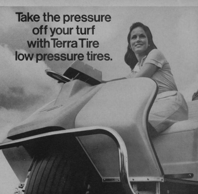
A fully loaded golf car with these flotation tires exerts only about eight pounds of pressure per square inch. Walking pressure under the heel of a shoe can be as much as 24 pounds per square inch.
