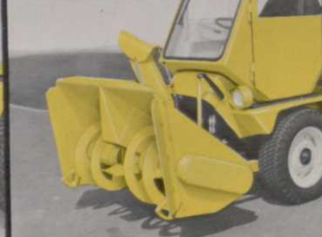
Two-stage snow caster, with 18" auger, clears 48" path
