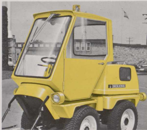
VEHICLE CAB Fiber-glass cab has all around visibility, removable doors, sliding glass windows.
