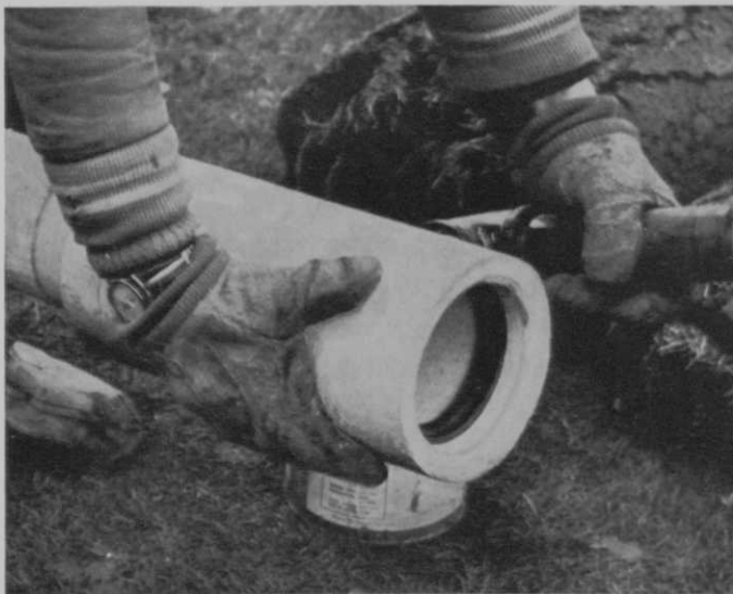
TRANSITE* asbestos-cement pipe with factory-mounted Ring-Tite tapped coupling for sprinkler riser. Rubber ring in precision-machined coupling speeds installation, provides tight flexible joint, reduces maintenance costs.
