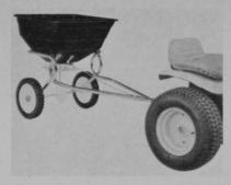
The F.D. Kees Mfg. Company introduces a pull model seeder and fertilizer. The P-54 Kees-Kaster has a non-corrosive hopper with a capacity of about 50 pounds of fertilizer. The frame and A-type hitch are made of plated tubular steel. Wheels are 10 inches. The Kees-Kaster can provide coverage over a 5-foot area.
