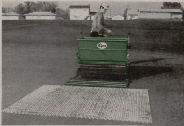
A large dragmat may be attached to do two operations at one time. Or, brushes may be added to the drag section for brushing in top dressing.
