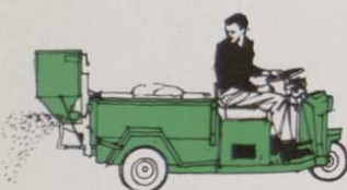
POWER TAKE-OFF SPREADS FERTILIZER
