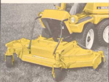
Rotary mower with 6 ft. cutting width
