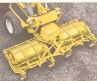
Reel mower cuts 10 ft. wide swath
