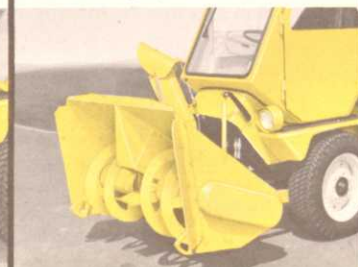
Two-stage snow caster, with 18" auger, clears 48" path
