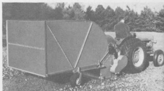
The GROUND'S GROOMER picks up thatch, clippings and debris in a 5-foot path.
