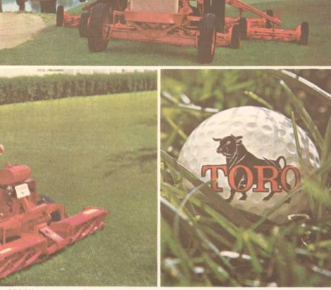
**70" Professional**<sup>®</sup> TORO'S all-around golf course mower...for approaches, tees and bunkers. Powered by a 6¼ hp., 4-cycle engine... cutting capacity over 14 acres a day. The three 25" reels are easily adjustable without tools to a height-of-cut range from ½ to 2½ inches. Equipped with large pneumatic turf tires which minimize compaction... and the Pro is exceptionally stable on hills due to low center of gravity.
