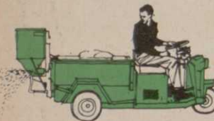
POWER TAKE-OFF SPREADS FERTILIZER
