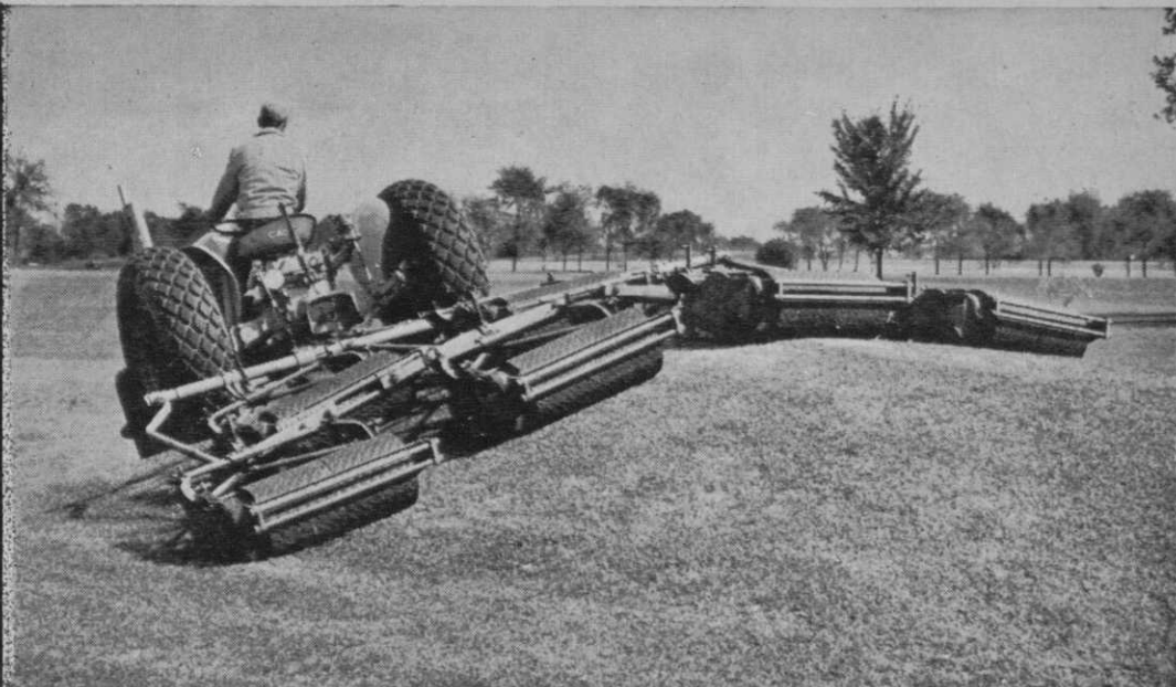
Roseman Mark IV Hi-Speed-Reel Hollow Roller Drive Fairway Mower
