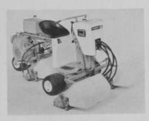
Jacobsen Manufacturing Company has recently announced the new riding triplex Greens King mower that cuts mowing time by two-thirds, says the company. It cuts a 62 inch swath, mows an entire green without having to run off for turning, and can cut 18 average-sized greens in three and a half to four hours.
